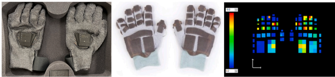
Fig. 1. The PPS tactile glove system utilized in this study.
